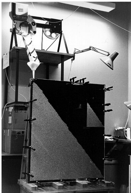
Figure 8: Experimental setup for investigating a self-organized rice-pile (courtesy Anders Malthe-Sørenssen).
