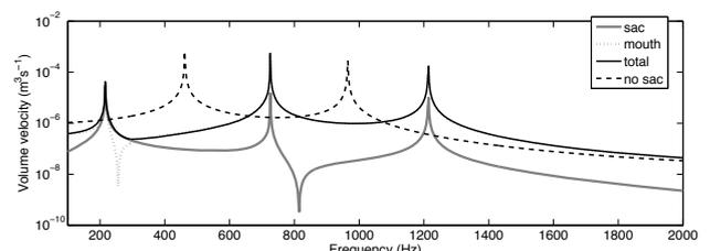
Fig. 5 Sound output spectra of the tract with air sac (and the contributions of sac and mouth separately) and the sound output of the tract without a sac.
