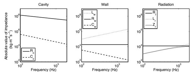
Fig. 2 Impedances for frequencies between 100 and 2000 Hertz for the different elements of the lumped element model.
