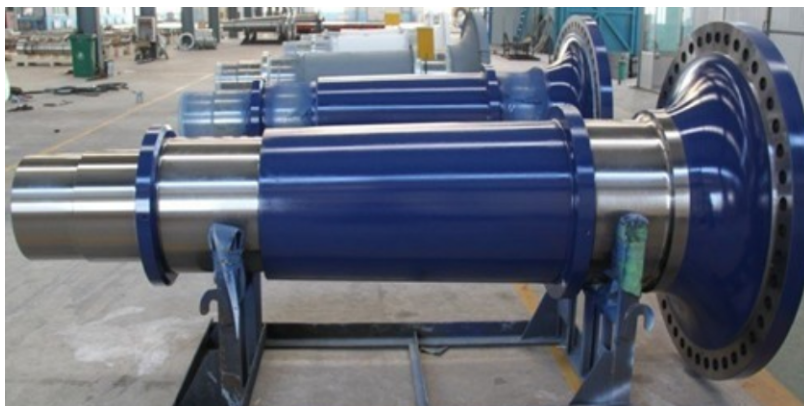
Figure 1.16: Several main/rotor shafts for wind turbines. Source: Fernandes [2023]
