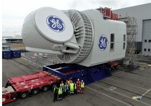
Figure 1.5: The nacelle of a Haliade X wind turbine. Source: Froese [2019]
