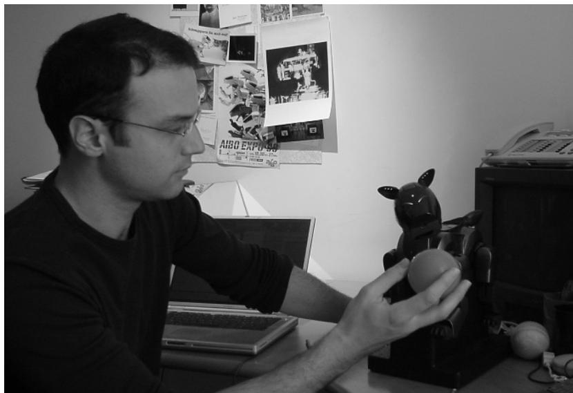
Figure 7.3: Our robot is an enhanced version of the commercially available AIBO. It is linked to an additional computer through a radio connection.
