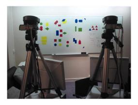
Fig. 2. The 'Talking Heads' experiment featured two pan-tilted cameras oriented towards a white board on which geometric figures were pasted. Agents used these cameras to play lexical games drawing attention to a chosen figure, which is the 'topic' of that game.
