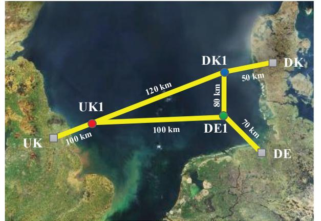
Fig. 6: The 6-node-meshed connected offshore MTdc network used in the simulations.
