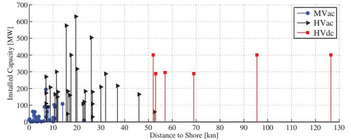
Fig. 1: Distance to shore, transmission technology and installed capacity of offshore wind projects [3].
