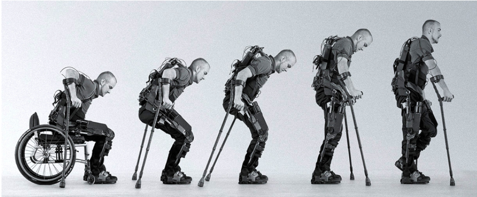
Figure 1.1: Agro’s ReWalk exoskeleton that supports paraplegics in everyday activities such as walking and standing up. (Medical Expo, 2014)
